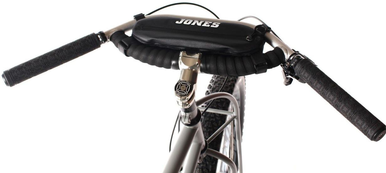
**Warning: All four (4) main straps must be secured around the tubes of the H-Bar at all times to ensure your safety. Make sure to check that the four (4) main straps are secure before each ride because they are critical for the pack's stability. Check your H-Bar Pack and its attachment straps for damage with every ride. If the H-Bar Pack is not attached correctly or is damaged it can come loose and get caught in your wheel causing serious injury.**
